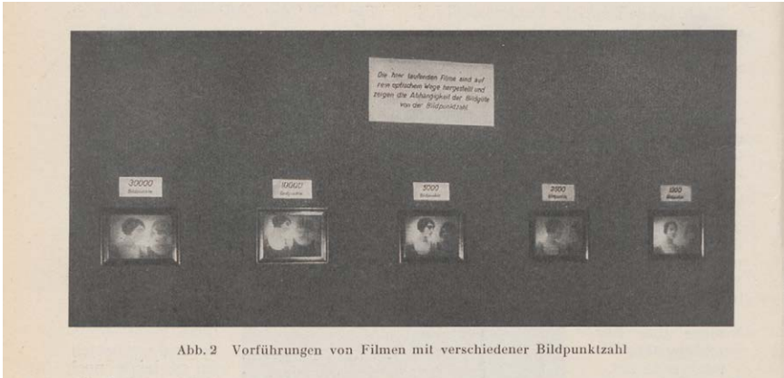
Fig. 6: A comparison of varying picture line counts. Images taken from the German magazine Fernsehen , 1931.
